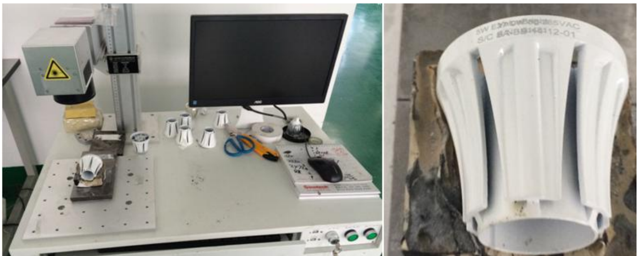
Laser silk-screen machine. This machine can print the logo, LED lamp parameter, model NO. etc. It is more professional.
