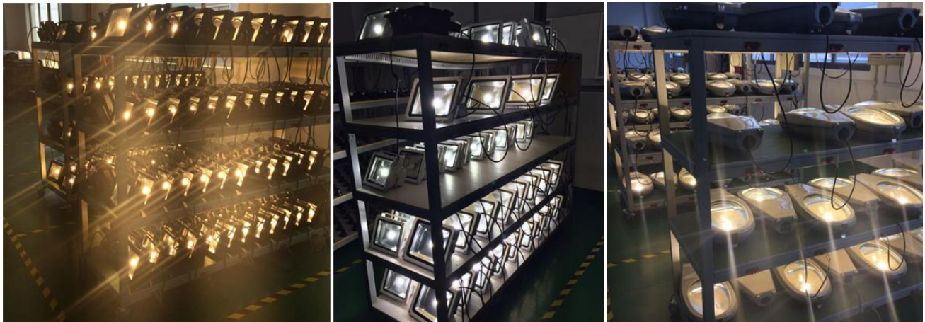
Aging Test. After safe test and lighting test, will be the aging test, aging test will last for 24 hours.
